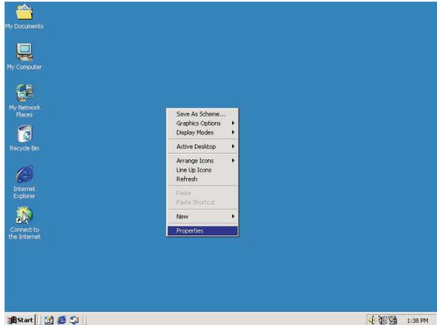
2. Select “Display Properties” → “Settings” so that you can adjust the parameters of the two monitors.
